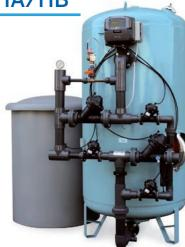
The tank is made of steel and it is protected internally by a food-grade layer of epoxy resins of controlled thickness and covered externally by a layer of enamel paint. The harness is in corrosion-proof PVC Noryl. Ultra Line HA softeners are available in tanks ranging from 500- to 1200-mm in diameter. For tanks with 950- to 1400-mm diameter it is available also a HB version, with larger harness, in order to facilitate higher service flow rates.
