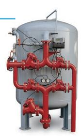
The tank is made of steel and it is protected internally by a food-grade layer of epoxy resins of controlled thickness and covered externally by a layer of enamel paint. The cycles are controlled by diaphragm valves, made of epoxy painted cast-iron. Ultra Line HB softeners are available in tanks ranging from 1500- to 2500-mm in diameter.
